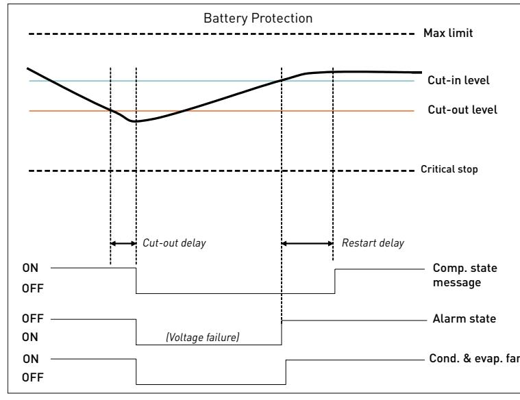
For initial startup after power ON, extra protection has been provided by allowing cut-in only when the voltage exceeds cut-out + 1 V DC.
